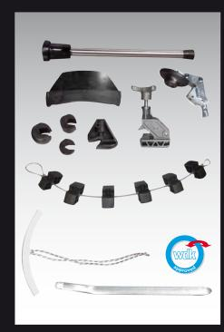
The plus kit is certified by wdk. It consists of plastic bead breaker disc, tyre lever plus, rod with tapered roll, plastic tyre protector, triangular bead pusher, spacers and plastic protector for bead breaker blade, Smart Bead Spacer and a bead clamp.
