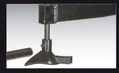
This hook is integrated in the bead press tool to easily lift heavy tyres during demounting and increase productivity.
