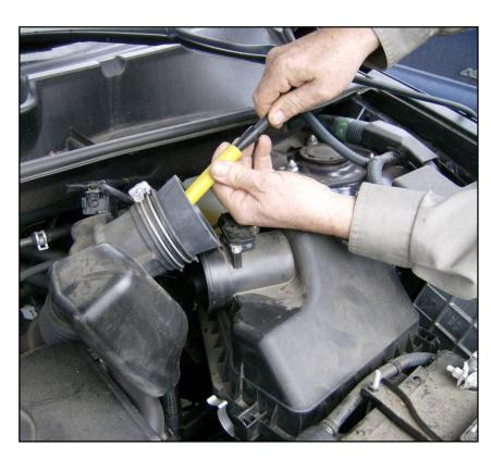
> Use cone to access intake system and connect smoke supply hose to cone.
