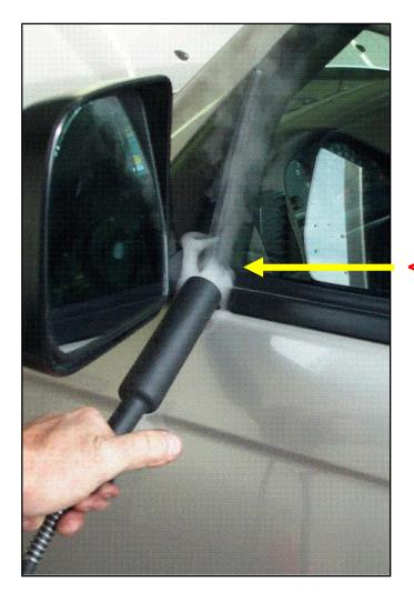
Smoke distrubance pinpoints the leak
