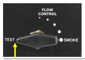
**TEST**: Delivers non-smoke air and a very accurate flow meter reading. This setting is for determining if a leak exists and how large it is.
