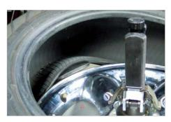
Demounting of the lower bead by means of the bead breaker disc. Fast and easy.
