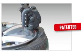
The integrated demounting finger supersedes the conventional tyre lever. It pulls the bead over the rim edge, being as gentle to the tyre as can be and and reducing the effort of the operator.
